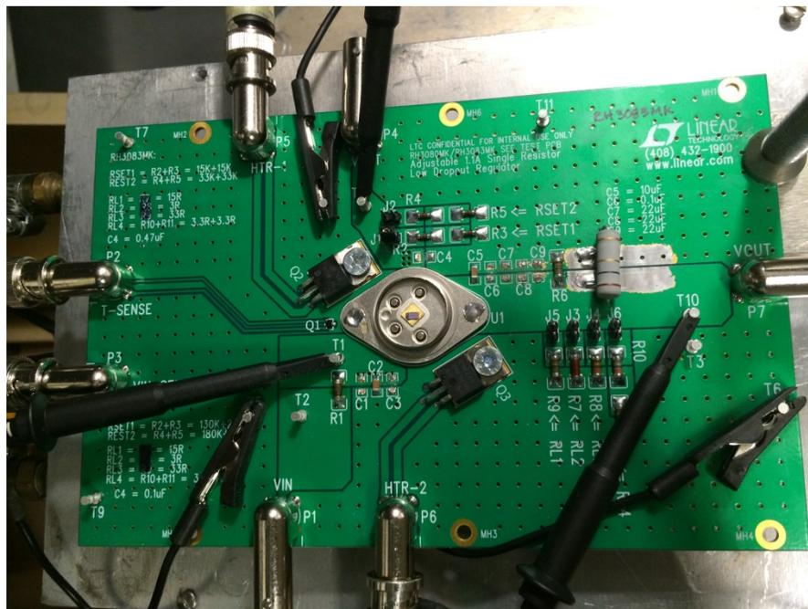
Figure 4a) Photograph of the RH3083MK SEE test board showing the exposed die. The cooling plated ended up not helping to dissipate heat due to a failing thermal conductive path from the test board to the cooling plate
