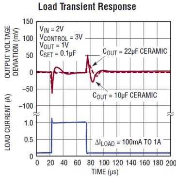
Fig. 6: Load Transient Response vs. Settling Time
