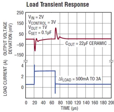
Fig. 7: Load Transient Response vs. Settling Time
