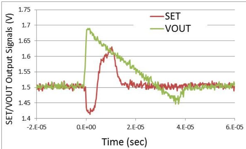
Fig. 10: Negative followed by Positive Transient Pulse on the SET signal vs. Beam Time Run 98, Waveform 84
