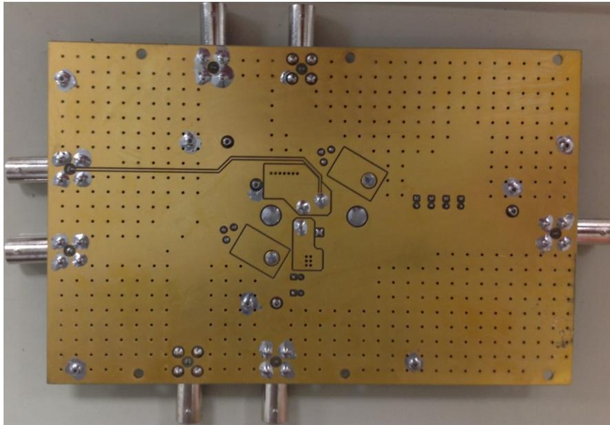
Figure 4b: Photograph of the bottom side of SEE test board showing the high number of Thermal Vias that were added to dissipate the heat through Conduction in the Heavy-Ion Vacuum Cell
