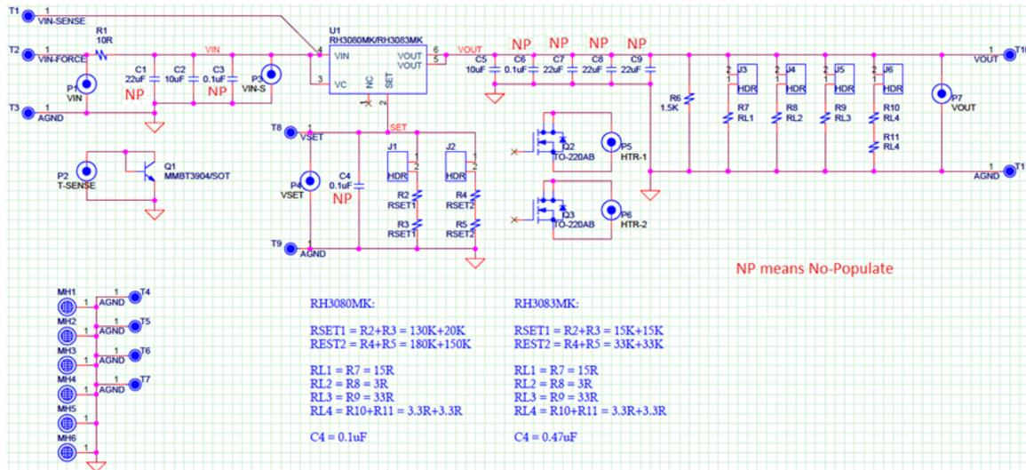
Figure 3: Block Diagram of the RH3083MK SEE Test Board\*
