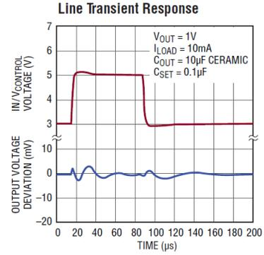
Fig. 8: Line Transient Response Time vs. Settling Time
