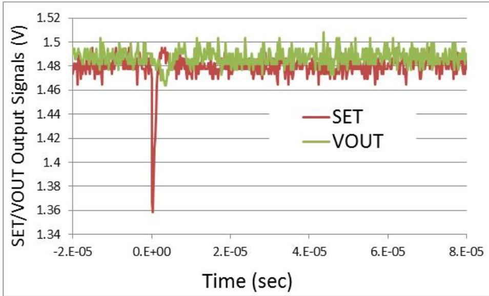
Fig. 9: Sharp Negative Transient Pulse on the SET signal vs. Beam Time Run 14, Waveform 3
