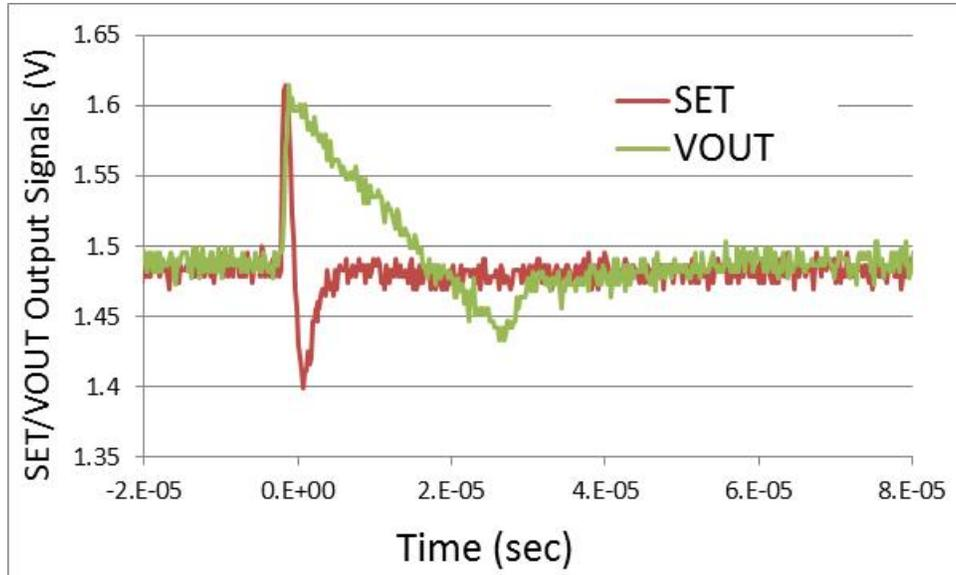
Fig. 13: Positive Pulse followed by Negative Transient Pulse on the SET signal vs. Beam Time Run 14, Waveform 6
