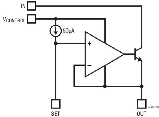
Figure 1: Block Diagram of the RH3083M DIE
