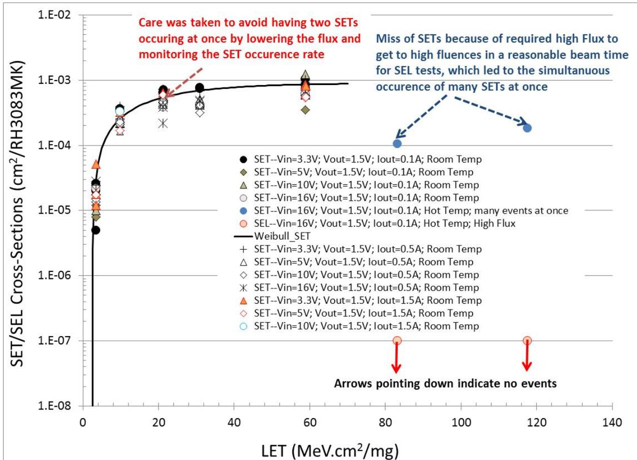
Fig. 17: Measured SET and SEL Cross-Sections vs. LET, showing:
