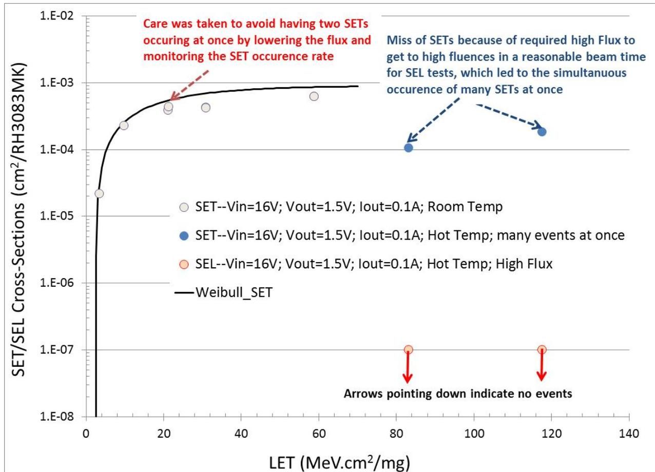
Fig. 18: Measured SEL Cross-Sections vs. LET, showing the RH3083MK immunity to Destructive Events and SELs. Arrows pointing down are indication of no observed SETs up to that fluence at tested LET
