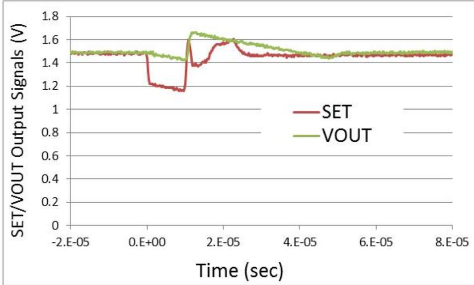
Fig. 11: Negative and Positive Transient Pulse on the SET signal vs. Beam Time Run 14, Waveform 102
