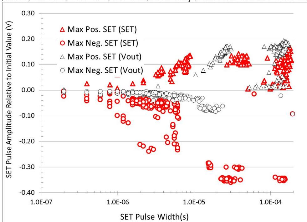
Fig. 16: % SET Pulse-Amplitudes vs. SET Pulse-Widths
