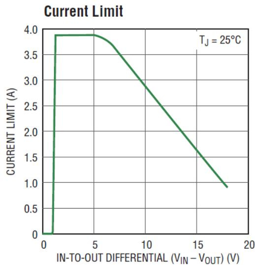
Figure 5: LT3083 Current Limit, extracted from LT3083 datasheet, Typical Performance Characteristics, page 6\*
