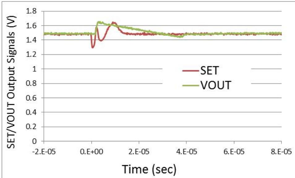
Fig. 12: Negative and Positive Transient Pulse on the SET signal vs. Beam Time Run 14, Waveform 4
